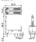
Marking Plate (integrated with release lever)
