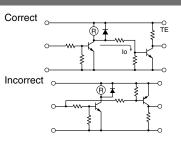
2-5. Surge suppression for transistor driving circuits:
