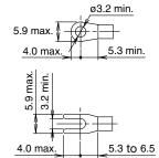
Note: Ring terminal cannot be used on SJ2S-0L.
