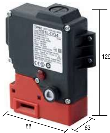
Conventional (HS1L): Volume 715 cm 3 Locking force 3000N
