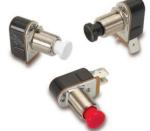
The P27-Series pushbutton switches are single pole, AC rated switches suitable for general purpose applications with a shallow back panel. These switches are momentary action with a medium actuation force (26 oz. typical). The P27-Series switch is equipped with a slow-make, slow-break contact mechanism, rated at 6 amps with a nylon concave pushbutton.
